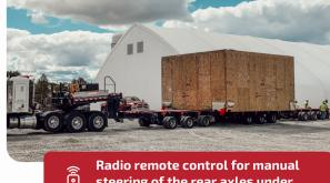
steering of the rear axles under limited conditions at low speed.
